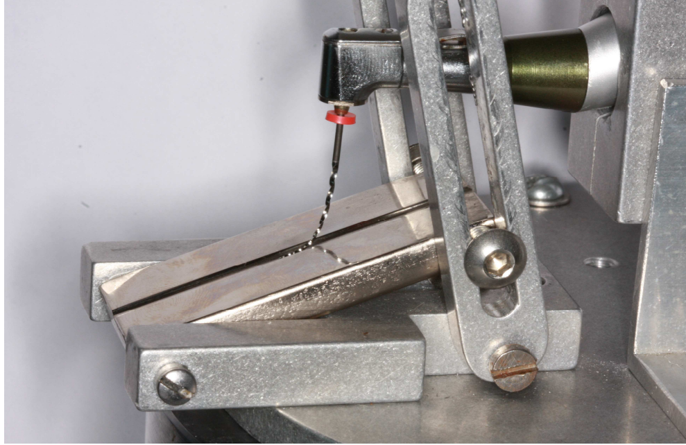
Figure 2: EndoSequence™ Rotary File 30/0.04 in Testing Apparatus
