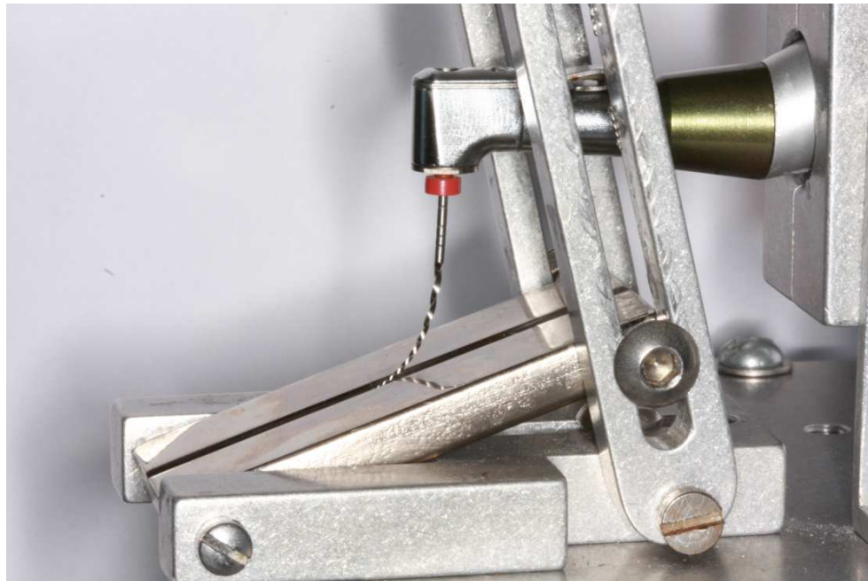
Figure 3: Profile® Vortex™ Rotary File 30/0.04 in Testing Apparatus
